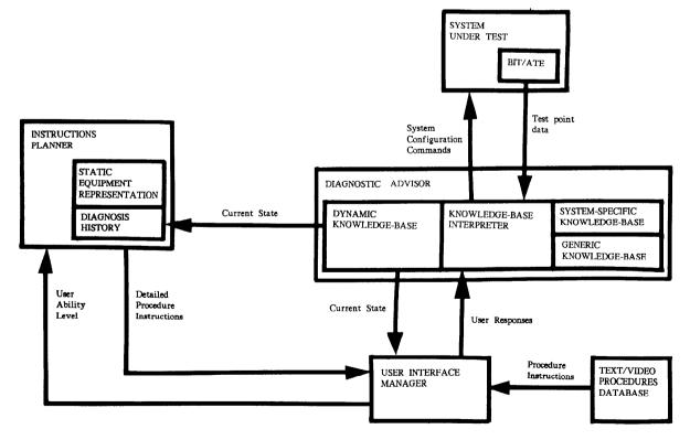
Figure 1. Architecture Diagram
