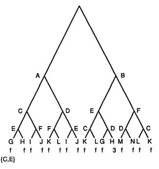
Figure 2: The search tree after labeling and dependency analysis. Capital letters are labels. The dependency set for the leftmost failure is also shown.
