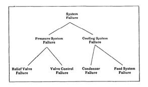
Figure 3: Hierarchy of malfunctions from Figure 1
