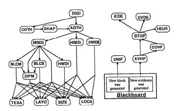
Figure 1. Dependency graph for specifying the temporal sequence of applying specialized tools.
