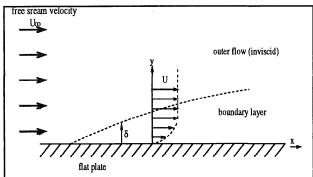
Figure 1: Boundary layer over a flat plate. The velocity gradient near the surface is large because of the no-slip condition. As one moves away from the surface, along the y-direction, the local velocity increases steadily as it approaches the free stream velocity.
