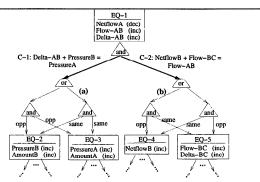
For each time-interval state, a chatter dependency graph is created describing the conditions under which each set of chatter equivalent variables can chatter with respect to the current state. In the figure, the qdir for each variable is displayed within the node. The AND-OR subgraph extending from an equivalency node  $EQ_{source}$  has the following structure:
