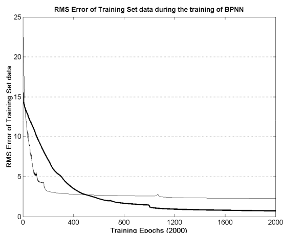
Figure 6 RMS Error of classification during training BPNN with the larger data set
