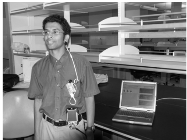
Figure 2: Person wearing sensors. The handheld computer is attached at the waist.
