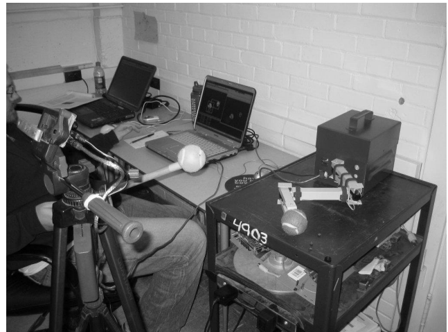
Figure 1: Narcissus is a three-link, planar, robotic arm. The tennis ball on the end of the arm is a color marker.
