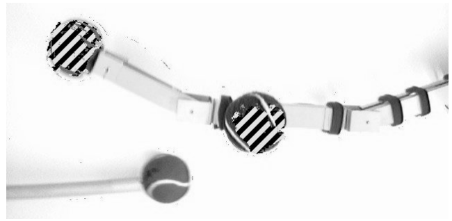
Figure 2: The cross-hatching indicates which color markers the robot considers “self.” Narcissus recognizes the red anticipatory distractor as “other.”
