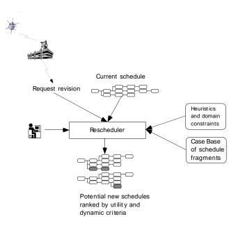
Figure 2: Operational diagram of ICARUS for rescheduling of the SCN
