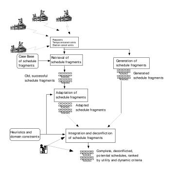
Figure 1: Operational diagram of ICARUS for normal scheduling of the SCN
