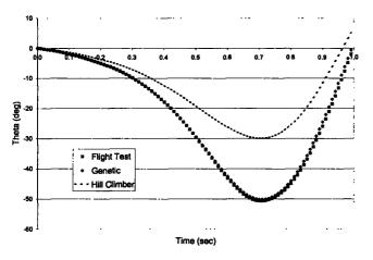
Figure 1. Euler Pitch Angle Comparison
