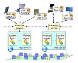
Figure 2: Architecture of the Agent-based OSA.
