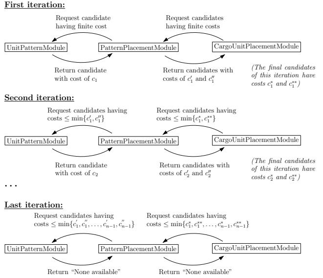
Figure 3: Communication of modules during optimisation.
