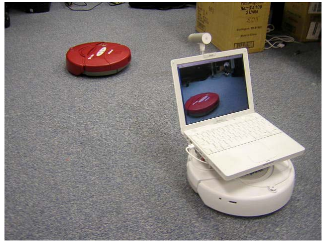
Figure 3a The Create chasing a Roomba Red based on color cues extracted from an onboard webcam, exhibited at AAAI 2007
