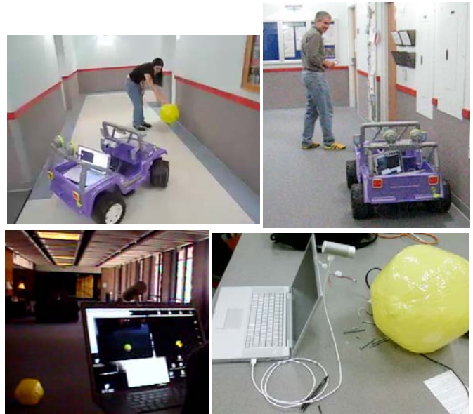
Figure 5 (top) Color tracking, and mistracking, using OpenCV. (bottom) Students with laptops – both Windows and Mac alike – are now able to prototype and test their software without the robot because OpenCV installs and compiles against student-developed code freely and easily. Porting to the robot involves nothing more than placing the laptop and the camera there.
