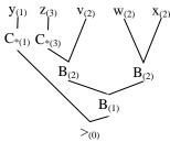
The normal form of the expression, after the  $\beta$ -reduction, is ((v (w (x y))) z) and can be represented by the following tree:
