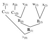
Again, we have a **B** combinator and the same rule applies. So, w level will eventually be reduced by 1. In addition, this **B** node has a sidling **B** node to the left, which means we have to add 1 level to the **B**, w and x nodes.
