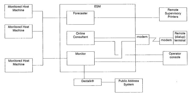
Figure 1. ESM System Architecture
