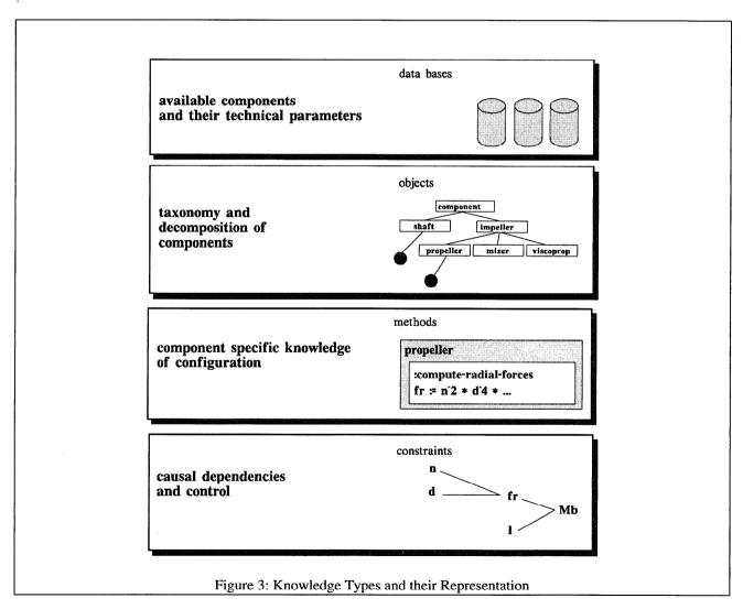
Second, the detailed mechanical design of the machine has to be determined. This is based on a constraint propagation.
