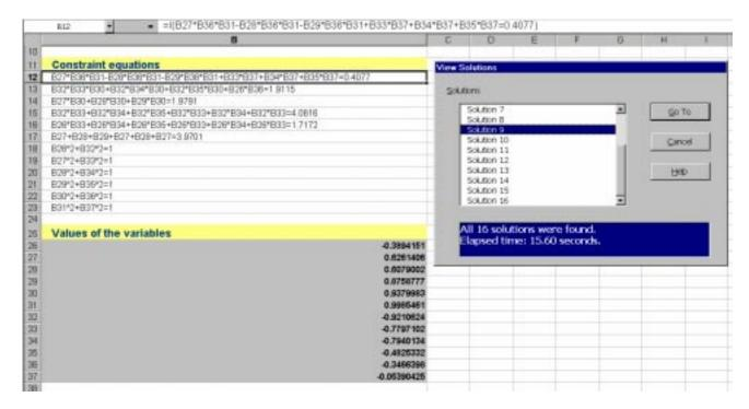
Figure 4. Finding all 16 solutions to kinematics equations describing a robot arm. The ninth solution is viewed.
