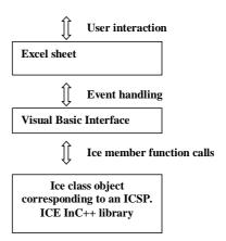
**Figure 6.** The interaction model of Interval Solver. Visual Basic interface layer catches user interactions (inserting data, moving cells, etc.) and commands. The Ice object, i.e., the ICSP corresponding to the sheet, is updated accordingly, or solved depending on the user interaction.
