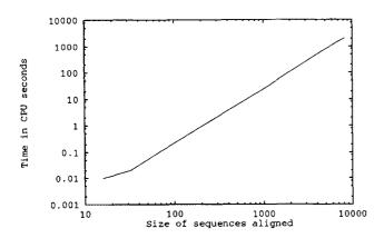
Figure 2: CPU time used by our heuristic to align pairs of equal length sequences on a Sun SPARC-10.
