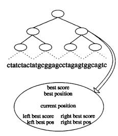
Figure 1: Data structure used to align the pattern within the text. In this picture, each leaf node represents 8 characters of the pattern, each of the internal nodes represents 16 characters of the pattern, and the root node represents the entire pattern. Each of the nodes contains the fields shown in the expanded node.
