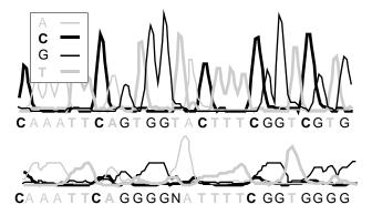
**Figure 5: Quality of Trace Data.** In the top sequence, the trace associated with each called base exhibits a sharp well-defined peak. The corresponding *Trace-Data Classifications* all show high *strong peak* scores. In contrast, the traces in the bottom sequence are flattened and overlapping; corresponding *strong peak* scores are generally nominal. The top sequence is much more reliable and is of high quality. We want to give the evidence it supplies more weight in consensus calculations.
