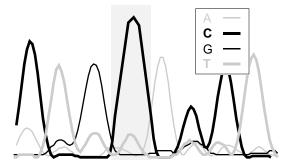
**Figure 4: Evidence in Traces.** Consider the evidence found in the four traces in the shaded region. The C trace will produce a high *strong peak* (SP) score, the T trace will yield a relatively smaller SP score, and both the A and G traces will produce valley scores. A visual examination of the traces supports the premise that the vast majority of the evidence is for a base call of C and that there is counter-evidence for a base call of A or G.
