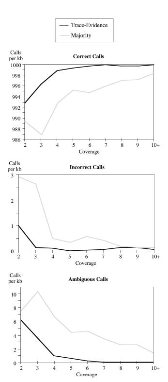
**Figure 10: Test Results.** Results for calls per kb vs. amount of coverage are graphed. Each data point is based on 20,000-68,000 consensus calls. The new *Trace-Evidence* method produces more correct calls and fewer incorrect and ambiguous calls, especially at low coverages.
