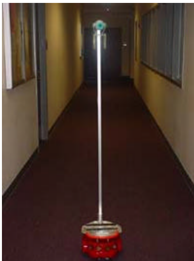
Figure 5: Cherry with platform and eye-level camera
