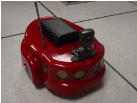
Figure 2: Lola featuring the antenna of the wireless modem, camera, and image transmitting device.
