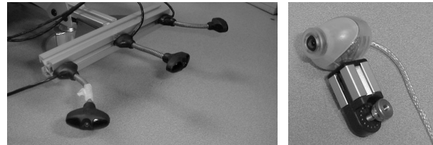
Figure 2: The three elliptical-beam IR sensors, which provide about 30" x 20" of coverage, and the irez webcam that are part of our ER1 configuration.
