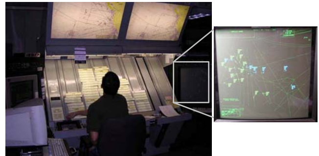
Fig. 7. U.S. Oceanic workstation with flight strips (center), sector maps (top) and spatial situational display (right) (from Major et al. 2004)
