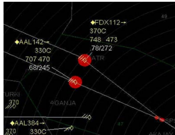
Fig. 5. An example of an aircraft conflict – the large red circles highlight aircraft targets and the small red circles illustrate the predicted point of conflict at the merge point
