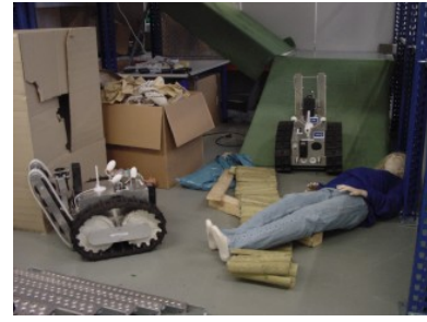
Figure 7: Two of the latest IUB rescue robots in a test scenario. The robots are normally tele-operated but they are also capable of full autonomy including the detection and localization of victims.
