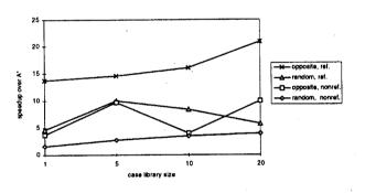
Figure 4: Mean speedup of SCBR algorithms over ground-level  $A^*$  (i.e., ratio of nodes expanded by ground-level  $A^*$  to those expanded by COVER) for refinable vs. nonrefinable abstraction hierarchies and random vs. opposite sides selection of start and goal positions. All abstraction hierarchies were created bottom-up.
