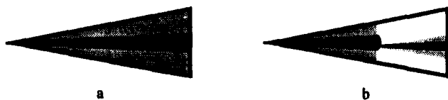
Figure 5: A standard exponential search (a) is transformed by a subgoal in (b), denoted by a black oval, into an initial search out to the subgoal, execution of that partial plan, then resumption of planning to the final goal.
