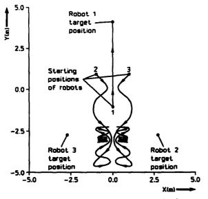
Figure 3: Trajectories of three congenial robots.
