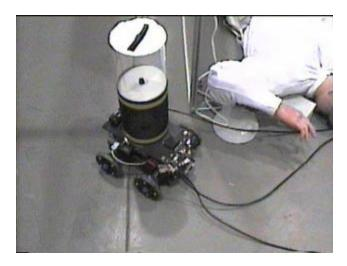
Cable control of the robot was chosen to avoid real-world problems of interference / loss of signal. When cable is used, it can become difficult to prevent it from tangling, especially if it's coiled. A common solution is to keep the cable as a figure-8, but this can be difficult to pre-stage and to transport. As a simple solution, we wrapped the cable around a piece of 3 in. PVC pipe about 2 ft. long using the pipe as a "kitestick," switching ends. The result is a figure-8 on the stick.
