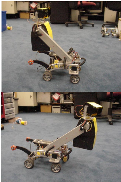
Figure 2: A moveable boom gives the rover a variable center of mass.
