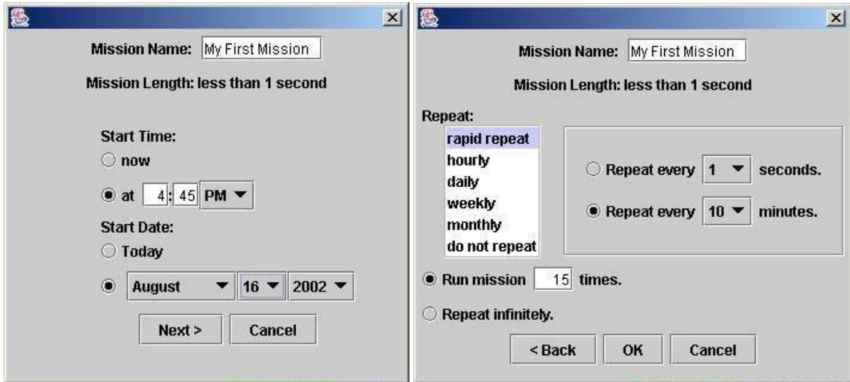
Fig 20: When scheduling a mission the user selects the start time and date as well as how often and how many times to repeat the mission.
