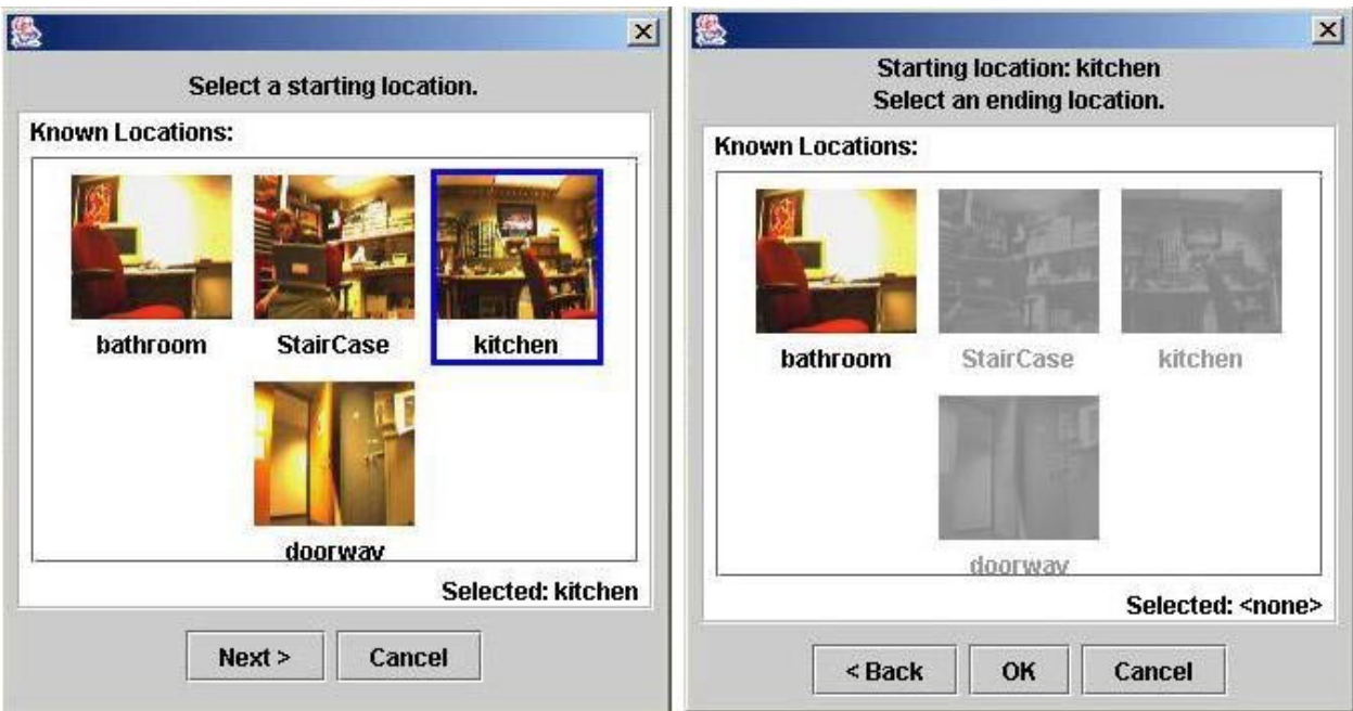
Fig 16: A popup window prompts the user to select a starting location and then an appropriate ending location to create a path. Ending locations which would create an invalid or unknown path are disabled.
