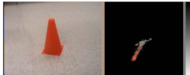
Figure 5. This image has the bright orange cone present, notice how the U and V visualization has grown to show that the particular color of orange is present in the image now.
