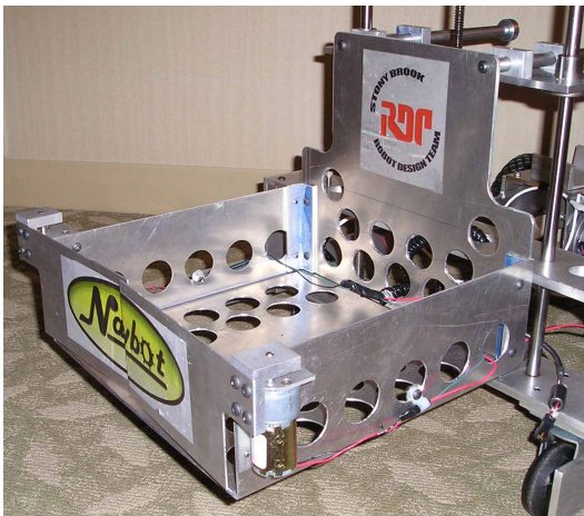
Figure 2: Linear vertical motion system of NavBot.
