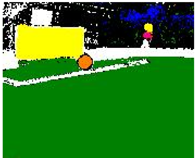
Figure 6: An example frame of video from the AIBO’s camera after color-segmentation post-processing.
