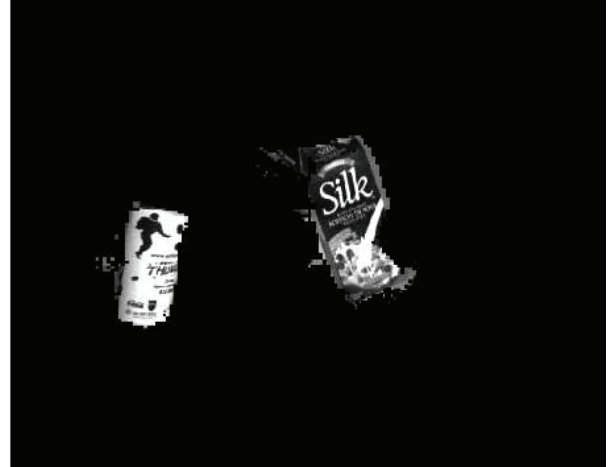
Figure 5: This figure shows the object snapshots of the cup and the milk box acquired through region voting.
