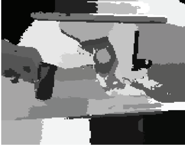
Figure 3: This is the resulting segmentation of the image and depth map in Figure 2 using normalized cuts based on both the pixel intensity and depth. Each region is represented by a constant gray level in this image.
