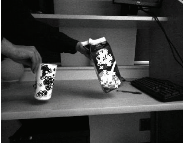
Figure 4: This image shows the position of two groups of rigidly moving image features from Figure 2. Rigidly moving features on the cup to the left are indicated with Os while rigidly moving features on the milk box to the right are indicated with Xs. Since the camera was static, there is no group of moving features associated with the background.
