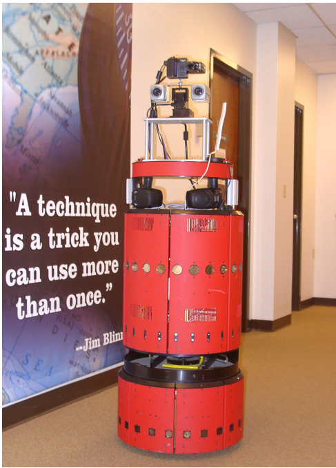
Figure 1: Lewis, our iRobot B21r research robot.
