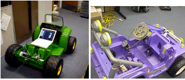
Figure 4 Two PowerWheels vehicles, adapted to run autonomously via an onboard laptop computer. Best suited for outdoor applications, these vehicles used vision, GPS, and sonar sensing in order to follow trails and navigate paths on campus.
