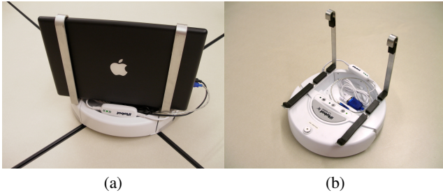
Figure 2: (a) Rear view of the MacBook mounted on the Create. (b) Create chassis with the MacBook removed, showing the aluminum mounting frame.
