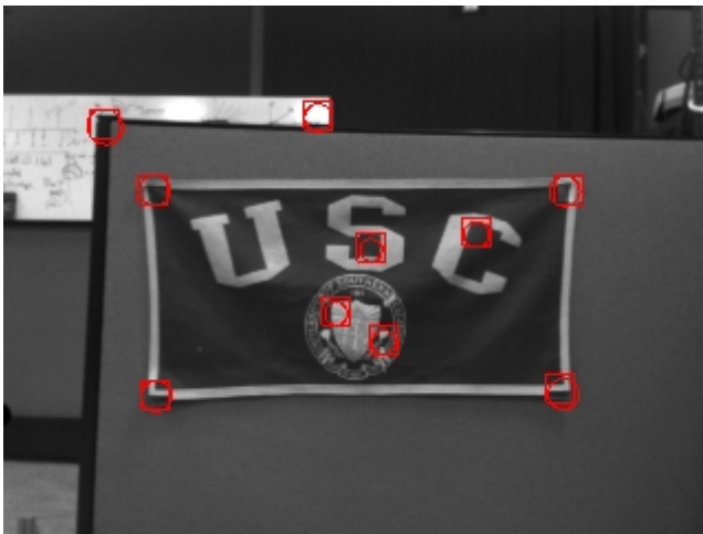
Figure 5: Image frame captured by the MacBook’s built-in iSight camera, showing features identified by MonoSLAM.
