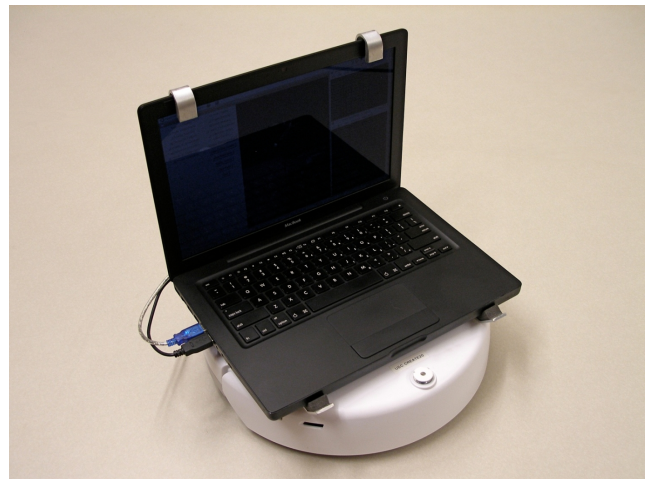
Figure 1: Apple MacBook laptop mounted on top of an iRobot Create. The MacBook provides exteroceptive and interoceptive sensors (a camera and an accelerometer, respectively), while the Create provides several proprioceptive sensors and the drive hardware for mobility. Together, they form a very capable robot platform.
