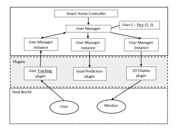
Figure 1. Illustration of an instanced data manager interacting with multiple plugins
