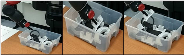
Figure 7: Robot using the pose estimated by the system to proceed with the part singulation task.
