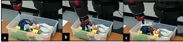
Figure 10: Robot using the pose estimated by the human to proceed with the part singulation task.
