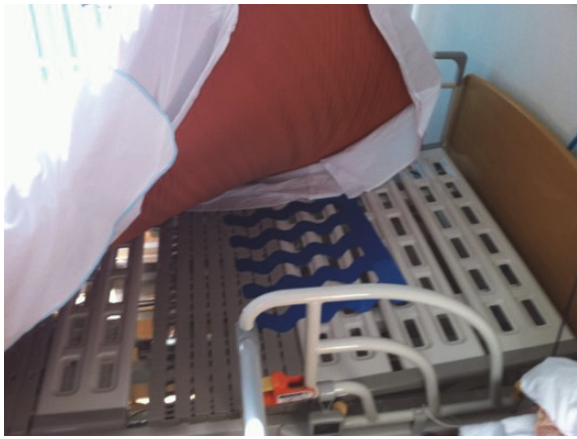
Figure 2: The EMFit sensor being laid under a bed mattress (the blue one in this image).
