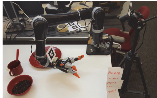
Figure 1: A typical manipulation pipeline combining multiple sensor streams. The fingers on the Jaco arm from Kinova contain proximity and force sensors and an Asus Xtion is used for depth and RGB imaging.
