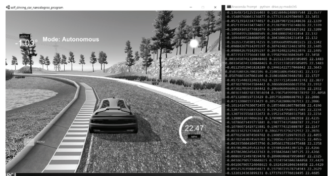
Fig. 4 The Unity Autonomous Car Driving Using Trained CNNs and Predicted Steering Angles
