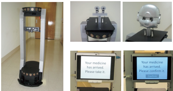
Figure 1. Basic PeopleBot platform (left). Additional humanoid features (right), clockwise from top left: abstract face; humanoid face; confirmation; and message only.
