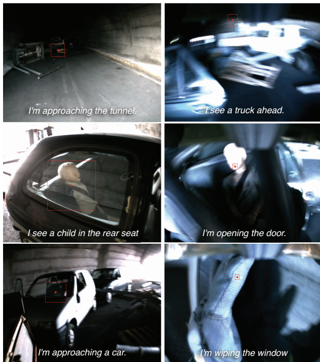
Figure 5: Fixations from the tunnel sequence labelled by the instructor running commentaries: these are examples of key frames used for action segmentation and to define compatibilities; the third figure above induce the constraint lookingAt(victim, t) during openingDoor(car, t') .
