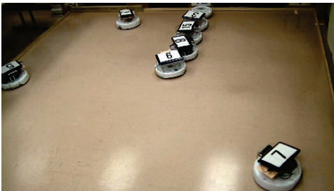
Figure 5: Snapshot of a ADDVERTEX operation. (Figure 4 shows this robot previously having spiralled to locate its nearest neighbor.)
