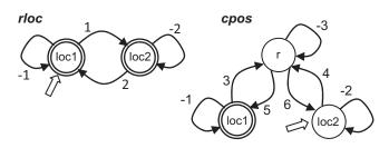
**Figure 4**. Representation of the planning domain (Figure 1) and problem using finite state automata with no-op actions.
