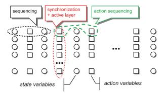
**Figure 6**. The structure of the constraint model, circles represent the state variables, squares represent the action variables.
