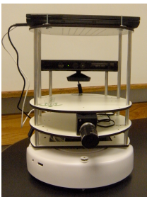
Figure 1. The Turtlebot with the Create base, the XBOX 360 Kinect, a small camera, and a laptop.
