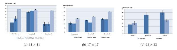
Figure 5: Interception times comparing proposed method (key events) to SARSOP low and SARSOP high precision. Our interception rates are comparable to those of high-precision SARSOP but we can continue to perform well even when maps are too large for SARSOP.
