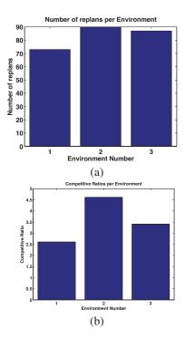
Figure 5: (a) Number of path replans done after encountering obstacles by the MRTA-RTPP algorithm for the three environments. (b) The competitive ratio of the path cost calculated by the MRTA-RTPP algorithm and the optimal path cost calculated offline with prior information of obstacles, for the three environments.
