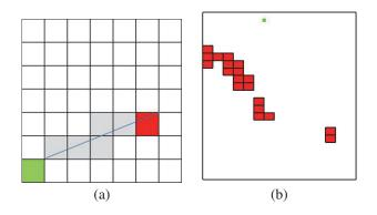
Figure 2: (a) Example for Bresenham line, (b) Obstacle grid map generated by Laser sensor
