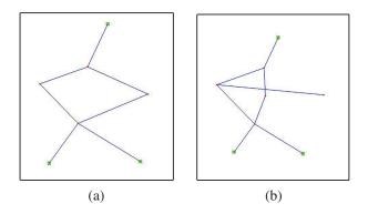
Figure 1: (a) Initially assigned paths to three waypoints (tasks) for three robots, (b) Updated path with newly added waypoints.
