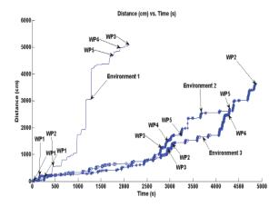
Figure 4: Time taken and distance traveled by a single robot to reach the set of five waypoints in the three different test environments.
