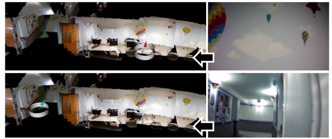
Figure 9. (left) The nine matches made during one of the autonomous "escape" runs by the drone out of the lab. The wider images were taken live by the drone; the narrower ones were taken a week before and used by RGBD-SLAM to build the 3d map of the lab below. (right) Two 3d renderings of the drone's position (frame 2 and frame 8) during the same escape run.
