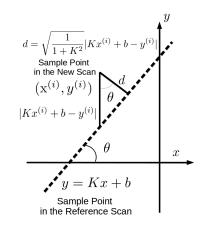
Figure 7: Perpendicular Distance for the Point away from the Line
