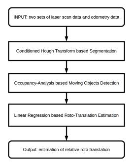
Figure 2: Overview of the Phases in Scan-matching Algorithm
